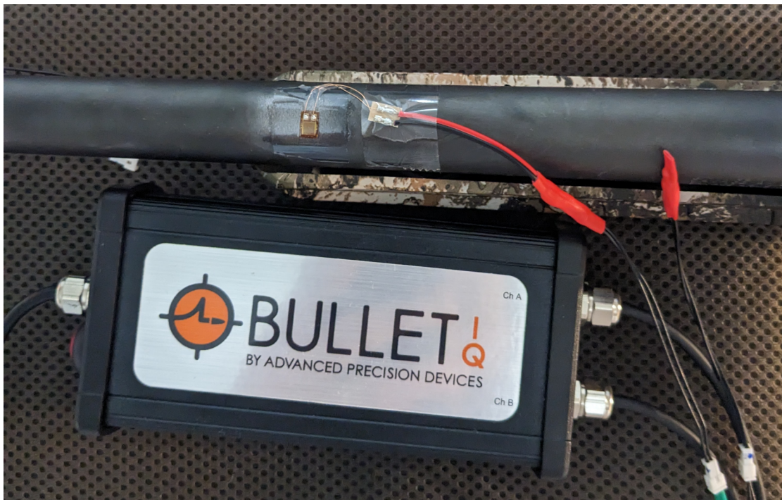
Figure 5: Applied gage and Completion Resistor (gage connected to green-indicated connector, and Completion Resistor on second connector)
